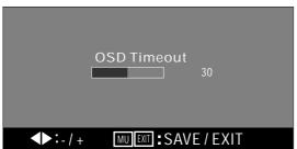
Press button 2: increase OSD timeout. Press button 3: reduce OSD timeout. Press button 1 to confirm setting. [Timout level: 10-60 . Preset:30 seconds]
